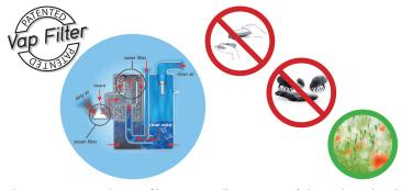
The VAP FILTER and water filter system allow savings of the traditional and expensive filters and bags. With steam are saved the costs of usage and disposal of detergents and solvents.
